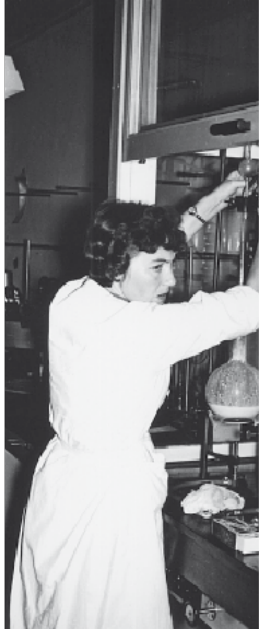
Laboratorieassistent (Technical Assistant) Klara Nordby destillerer ostprøver for analyse av flyktige forbindelser. Distillation of cheese samples for analysing volatile components.
