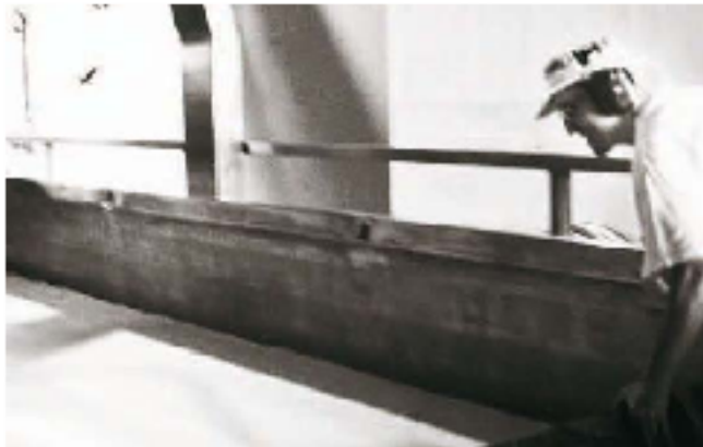
Collecting the cheese mass in a pressing vat before moulding. Elmesvågen Dairy.
