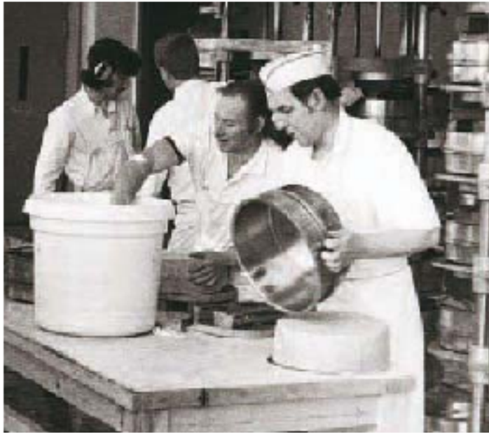
Traditional procedure in moulding cheese, using cheese cloths and moulds of stainless steel. Here removing of cloths.
